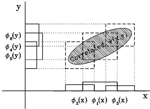
FIG. 1. Approximating a correlated wave function  $\Psi(x, y)$  by a sum of products  $\phi_j(x)\phi_l(y)$ . The rectangles on the axes symbolize the individual  $\phi$ 's, and the dashed rectangles indicate the support of a single product. Several products are needed to cover the non-aligned support of  $\Psi$ .
